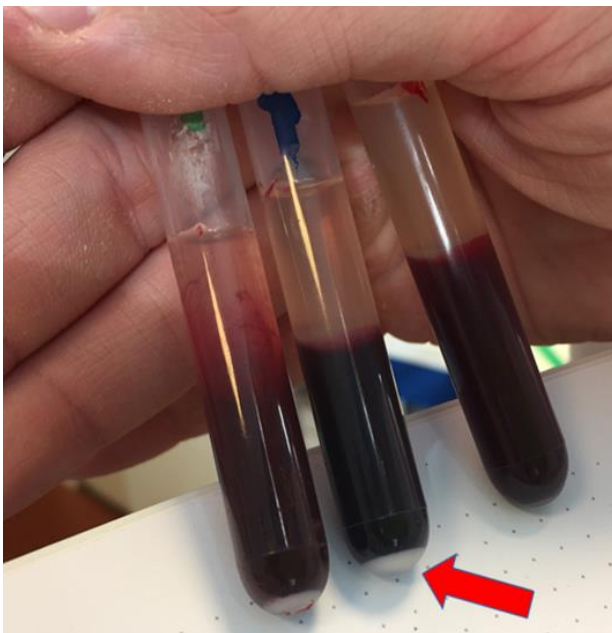
Figure 11. Two glass containers on left show precipitation of nanocapsules.
